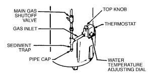
FIGURE 4-GAS PIPING AND DIRT LEG INSTALLATION
